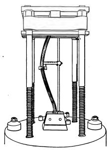
Fig. 52.—Method of testing buggy spokes.
